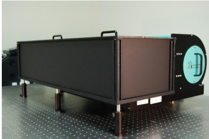
Figure 1: The High Output Temperature IRSP in a bench top collimator configuration
