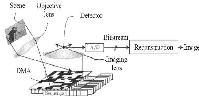
Figure 1. Single-pixel detector based multispectral compressive sensor
