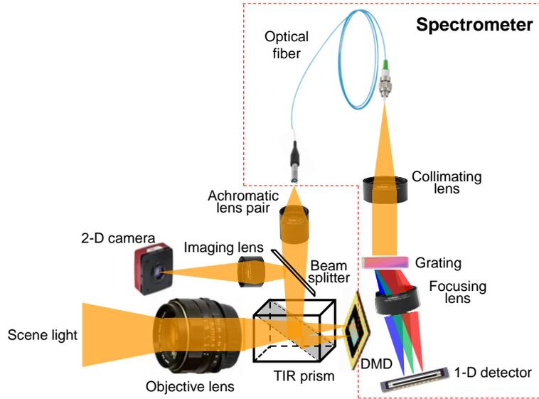
Figure 2. Schematic illustration of the 1<sup>st</sup> design of the compressive multispectral and hyperspectral sensor (CMHS) system.
